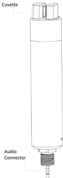
The BroadSensor UV254 sensor is an optical-based absorption and transmittance with UV LED and PD technology sensor. The sensor measures the absorption at 254nm and 550nm at the same time to compensate the SAC measurement for interferences from turbidity and color.
