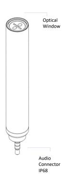
Broadsensor measures turbidity with an fiber optics sensor. An 860nm light from the emitter enters the sample via fiber and scatters off particles in the water. The scattered light at 90 degrees, enters a PD detector via fiber. This follows the nephelometric technique of measurement, and values are expressed in nephelometric turbidity units (NTUs). It follows the ISO7027 standard.
