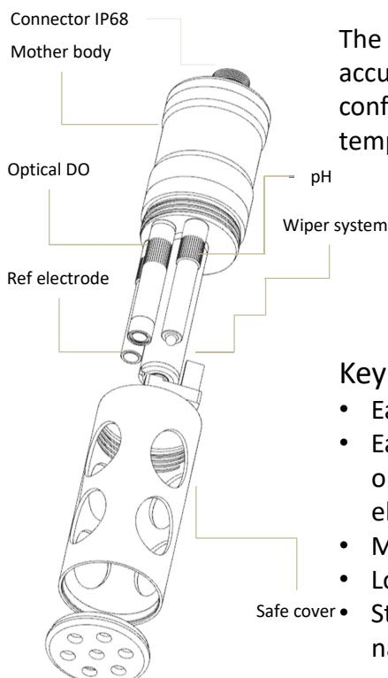
The AQUA200 water platform is rugged in aquaculture water, delivering accurate, reliable data in an easy-to-use for end fisherman. Base sonde configuration includes optical dissolved oxygen(optical DO), pH, ORP, temperature and wiper system.
