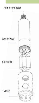
Broadsensor online ISE (NH4+ pH ORP/K+) sensor with integrated digital electronics for plug and play capability with Broadsensor multi-parameter sonde platform and IP68 connector to any PLC or RTU.
