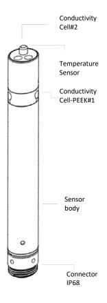
Broadsensor conductivity sensor measures conductivity by AC voltage applied to nickel electrodes inside of PEEK conductivity cell. The sensor require littles maintenance or special attention for storage and can measure high conductivity water long-term.
