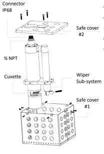
0000 0000 0000 0000 0000 0000 The Broadsensor UV254 sensor is an optical-based absorption and transmittance with UV LED and PD technology sensor. The sensor measures the absorption at 254nm and 550nm at the same time to compensate the SAC measurement for interferences from turbidity and color.
